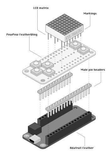
Make sure to insert the LED Matrix in correct orientation – with the markings in the same direction as the "down" button. Otherwise the colors will be wrong, and the image will be flipped.
